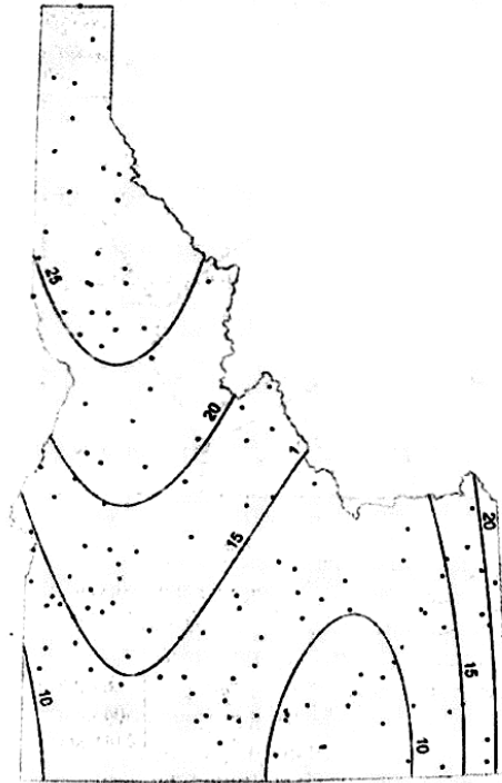
Fig. : An isohyet map in inches from a third-order trend surface model. The point symbols represent known points within Idaho.
