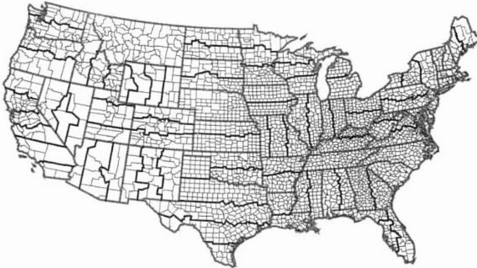
Fig. 1 : SPC83 zones in the conterminous United States. The thinner lines are county boundaries, and the bold lines are state boundaries. This map corresponds to the SPC83 table on the inside of this book's back cover.
